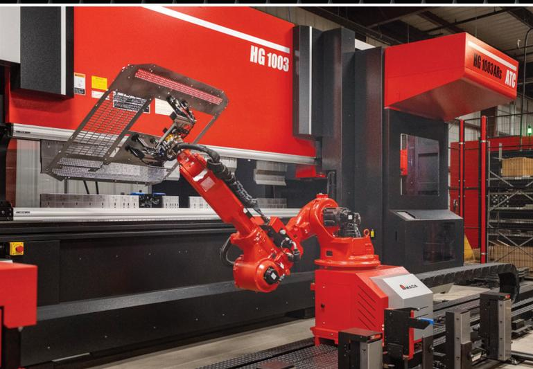
The HG 1003 ARs is designed to handle sheets up to 39" x 31" and the system's robot can support loads up to 44 lbs.
