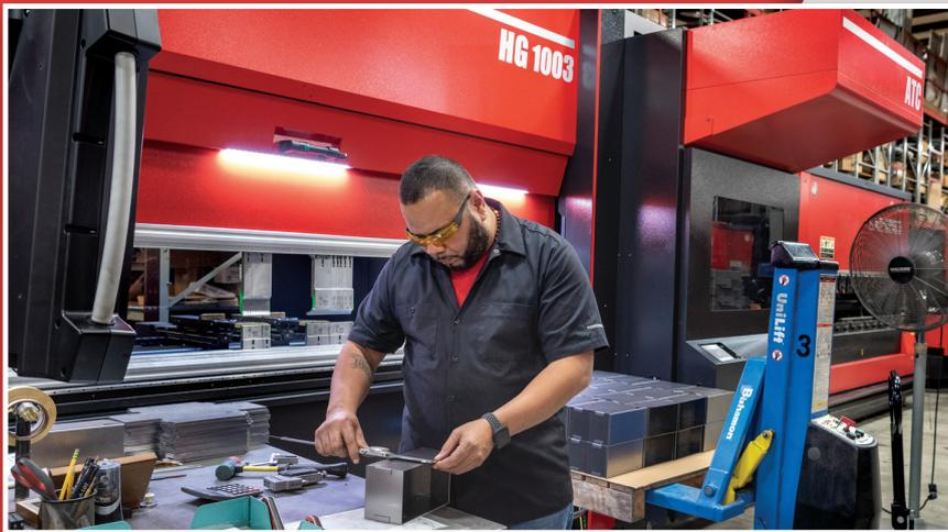
(Above: HG 1003 ATC) Complex bending is greatly simplified by the AMNC 3i control. The control and the Automatic Tool Changer (ATC) work together to make certain all tools can be staged at the same time. As a result, Vernier's operators can run more jobs in a single setup to optimize throughput.
