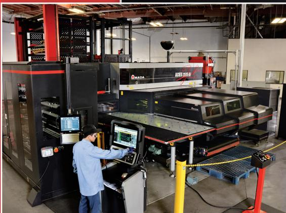
The ACIES 2515 AJ achieves continuous processing through automated tool changes and automated material handling — including single part removal and stacking.
